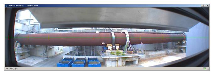
Application Example: View of built-in miniature IP-camera trough the scanner entrance window
