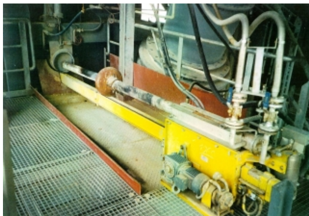
Fig.: Gas sampling probe with retraction device
